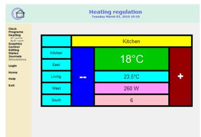
In this implementation, each room has ist own view, identified by the top caption and selected in the left column. The temperature set point, in the light blue central rectangle, can be modified by clicking within the large plus/minus boxes.
