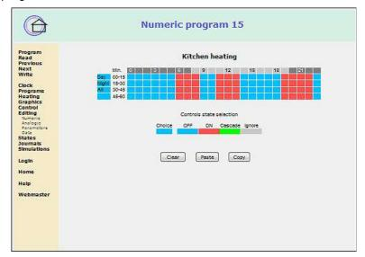
A **numeric program** is a time-of-day ordered list of values that are used to set numeric outputs or to compare with numeric inputs all along a day. This function is modelled on the standard electro-mechanical timer shown below.
