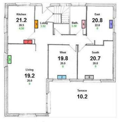
Assume a house with a living room, three bedrooms and a kitchen, all equipped with electric heaters. You want to have an independent temperature regulation system for each room.
